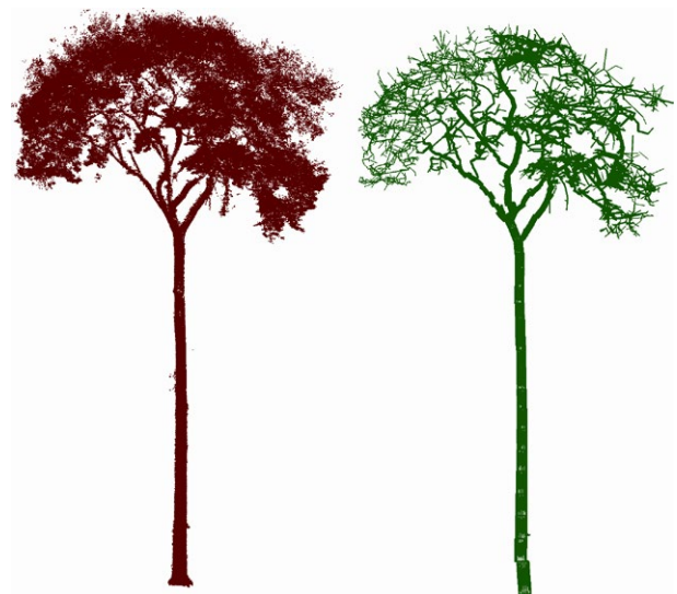
FIGURE 2 Example of one tree terrestrial laser scanning point cloud from Guyana dataset (left, in dark red), and the same tree modelled by quantitative structure models (right, in green). Figure from Gonzalez de Tanago et al. (2016)
